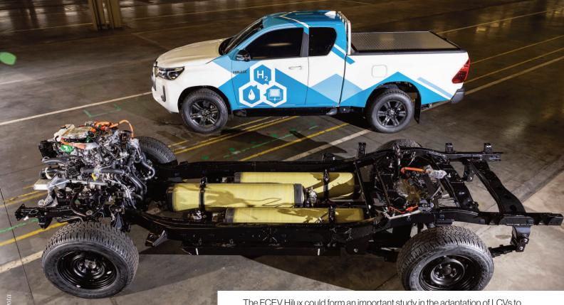
The FCEV Hilux could form an important study in the adaptation of LCVs to meet fleet operators' zero-emission goals (Photo: RKP Photography)
