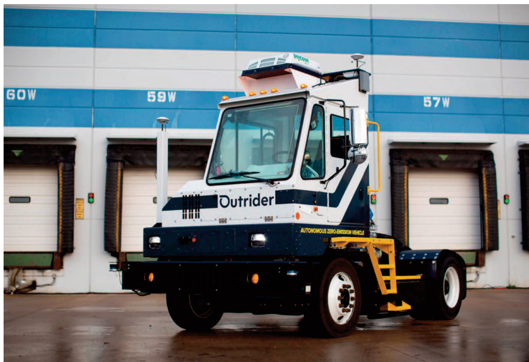
Outrider's vehicles can couple tractor to trailer and manoeuvre between dock doors, parking spots, and areas for over-the-road pickup
