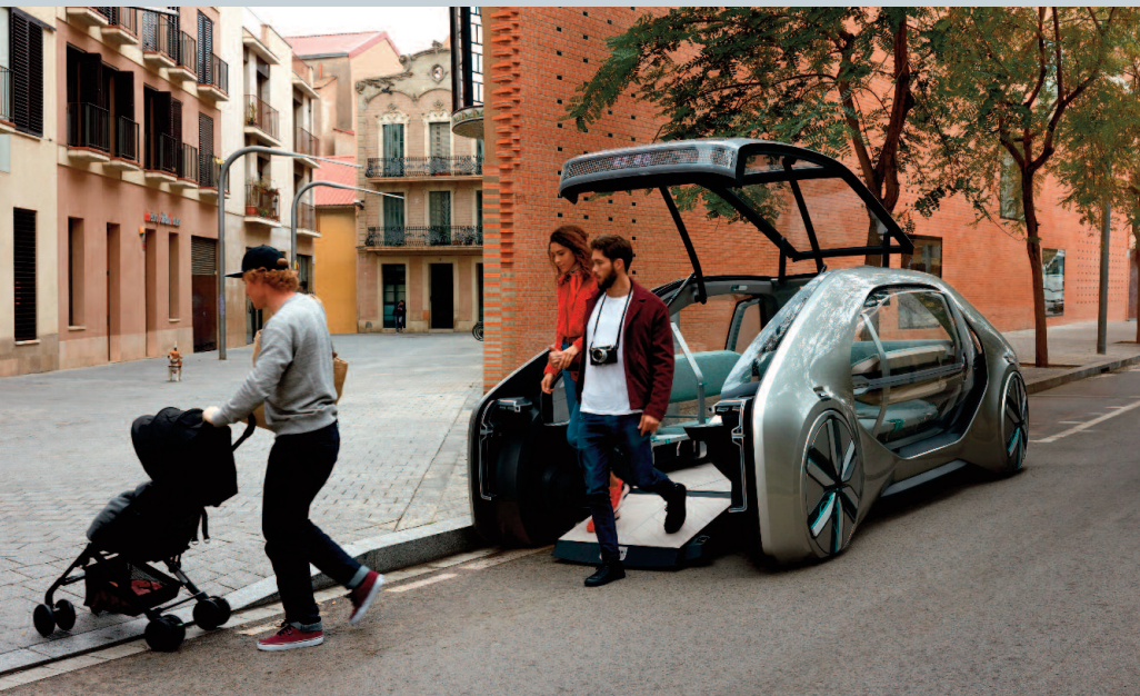
A purpose-built urban robotaxi, the Renault EZ-GO concept unveiled in 2018 is boarded via a large central 'hatch' at the front of the vehicle, and features a U-shaped seating arrangement
