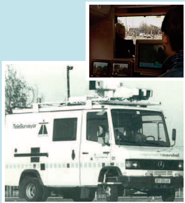
From small things... The first Tele Atlas road mapping vehicle was a Mercedes-Benz van loaded with 1,000kg worth of electronics equipment to capture and store pictures
