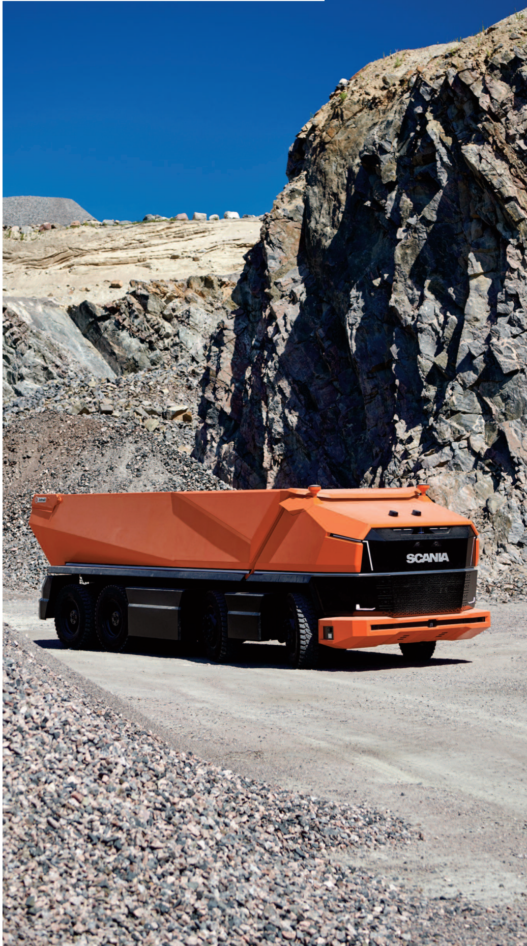
The Scania AXL fully autonomous cab-less concept truck uses a combustion engine powered by renewable biofuel
