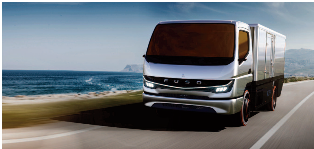
Daimler’s Fuso brand unveiled its ‘Vision F-Cell’ concept at the 2019 Tokyo Motor Show. A fuel cell range extender gives the truck a range of 300km
