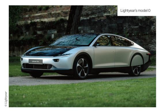
range (560km) than the Tesla Model 3 (16.1kWh per 100km and 360km respectively). More impressively, based on a 35km commuting route in the Netherlands, the Lightyear 0 was found to last two months between charges. Furthermore, this interval grew to seven months when tested over the same distance in the sunnier climate of Portugal.
